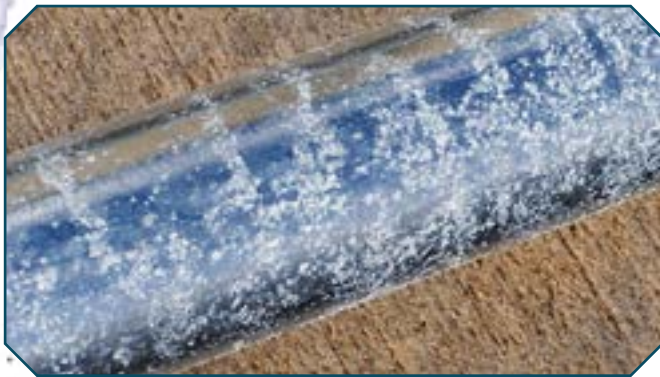
Figure 8: Medium wet storage stain
